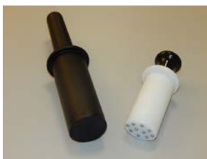
Figure 5: Standard pusher and rotating pusher
