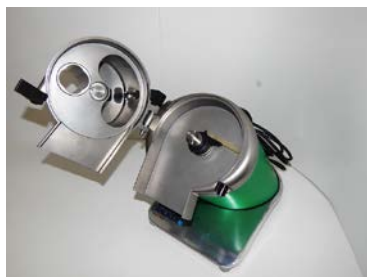
Figure 12: Assembling the ejector
