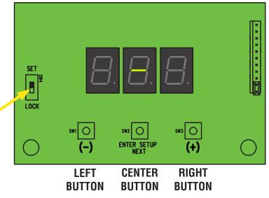
Switch must be in "SET" position for access into programming modes.
