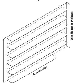
3. Install rack sides into existing holes inside the unit with thumb screws.
