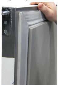
4. Place a white spacer on the bottom hinge pin.
