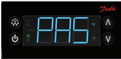
3. Scroll to **187** using the up/down arrows and push the stand-by button (lower left button) to enter.
