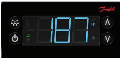
4. Scroll to **dis** using the up/down arrows and push the stand-by button (lower left button) to enter into the display menu.
