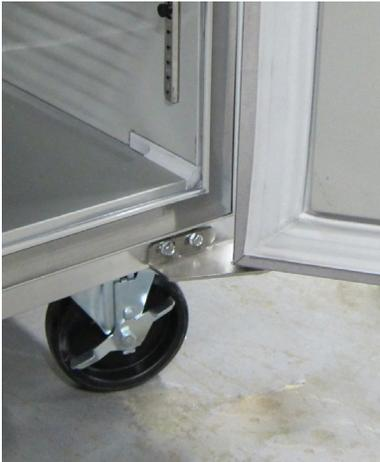
9. Check the door alignment. Check that it shuts and seals. Adjust the bottom hinge if necessary.
