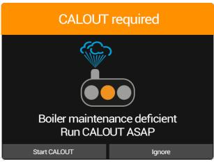
If you do not perform **CALOUT** by the end of the day, the next day the following popup appears: "Boiler maintenance needed, perform **CALOUT** as soon as possible." Press "Start CALOUT" (see next paragraph) to immediately perform **CALOUT** or press "Ignore" to perform the procedure later (example: at the end of the day).
