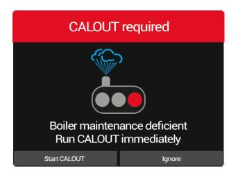
If CALOUT is not performed, once the maximum maintenance interval is reach, the following popup appears: "Boiler maintenance needed, perform CALOUT immediately."
