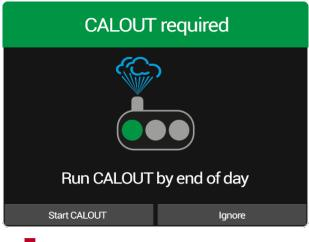
When the **CALOUT** process is needed, a popup warning appears: "Perform CALOUT by the end of the day". Press "Start CALOUT" (see next paragraph) to immediately perform **CALOUT** or press "Ignore" to perform the procedure later (example: at the end of the day).
