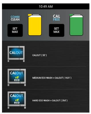
Select **CALOUT** or the desired **wash** + **CALOUT** and the washing procedure starts.
