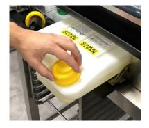
Remove the top of the new cartridge.
