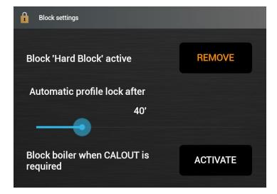
When the automatic lock has been enabled, drag the cursor to set the time after which the lock will be enabled.
