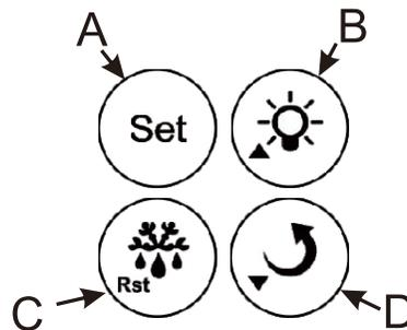
“D1” then press “A” button to enter the settings and change the settings to “00” and confirm by pressing “A” and the alarm is canceled. It will bring you back do “D1”. You need to go up to the settings “C1”.
