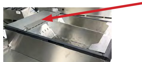
Incorrect placement of the food tray. Food tray is rotated 180°.
