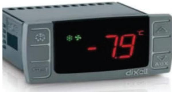
(1) To change temperature set point: Press & hold "SET" for 2 seconds until a flashing number appears in display, then release "SET".
