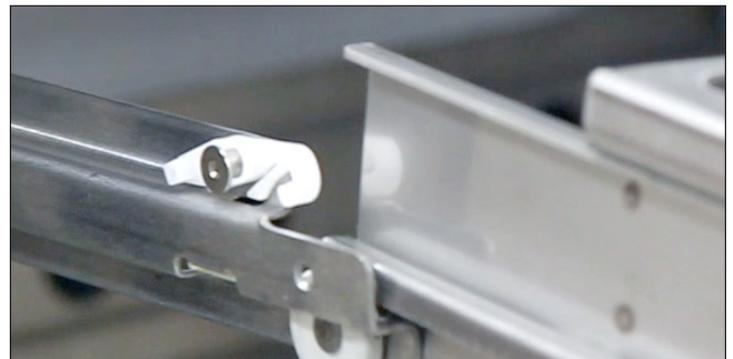
**Fig. 3.** Align the drawer with the drawer slide.
