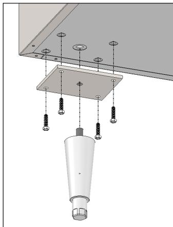
**Fig. 1.** Install the mounting plate and leveling leg.
